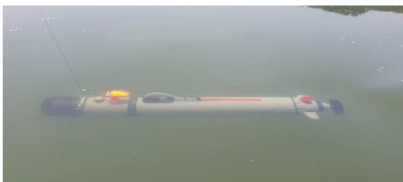
AUV under development: way point tracking test
