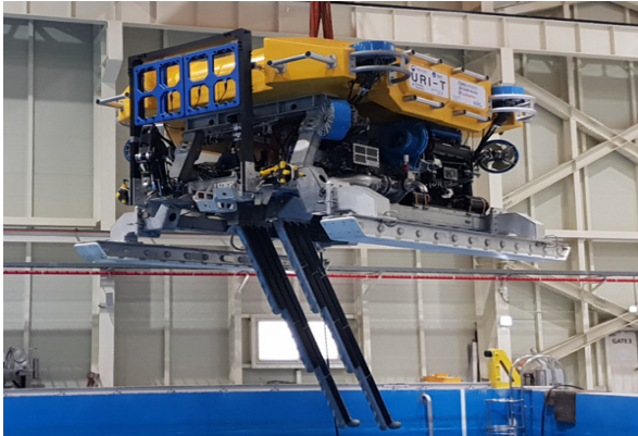
URI-T, an underwater cable burying ROV
