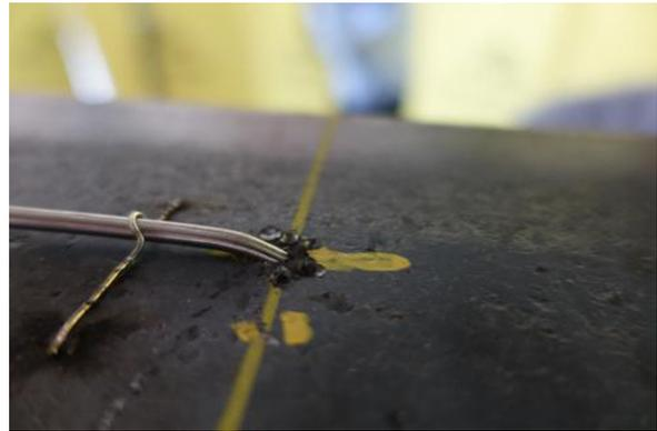
(b) Thermocouple for steel surface temperature measurement
