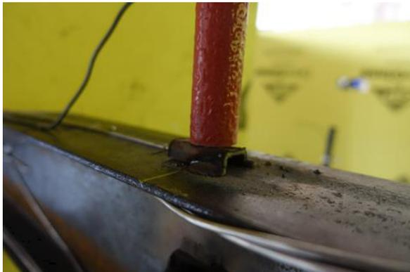
(c) Instrumentation for vertical displacement measurement
