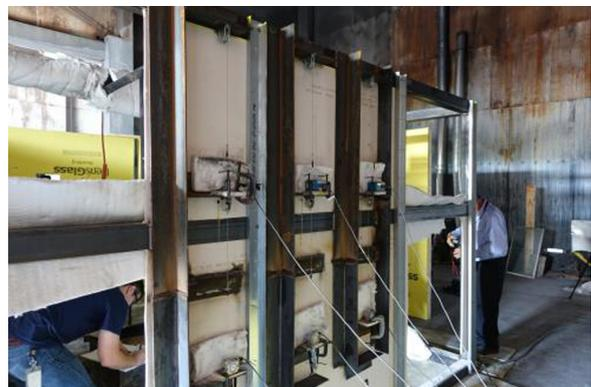
(f) String potentiometer for displacement measurement
