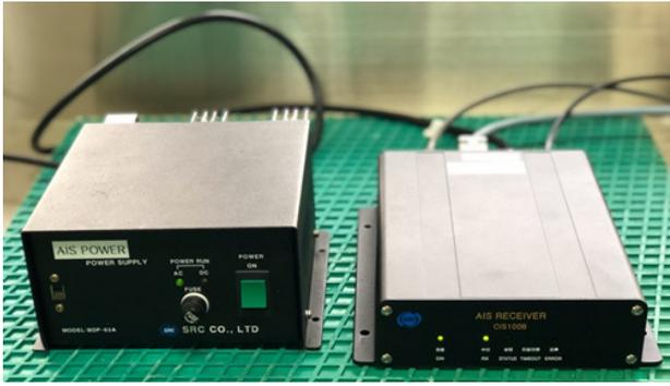
Fig. 1 AIS Receiver used by the proposed system
