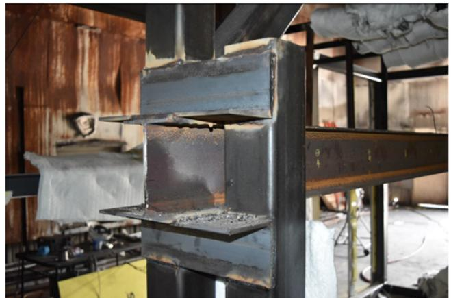
Fig. 4 Fixed end of specimen welded along all edges of both flanges
