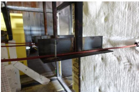
(e) Support for horizontal displacement measurement
