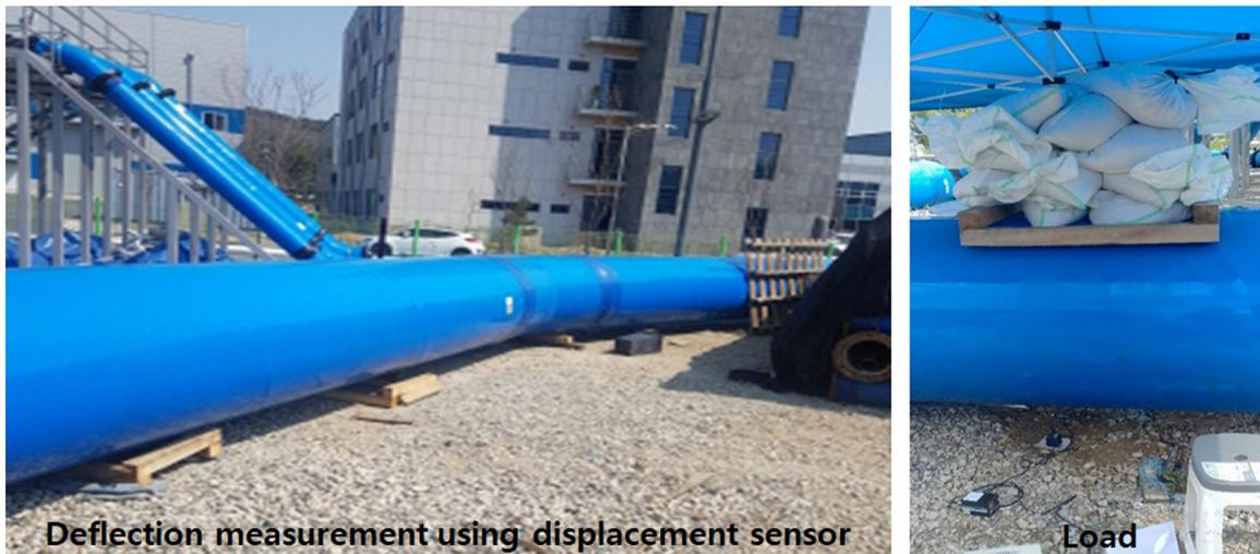
Fig. 6 picture of Load testing using sandbag and monitoring system using displacement sensor at exposed pipeline
