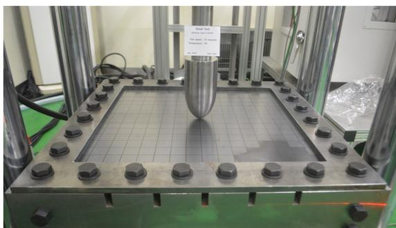
(b) Photo of a punch test for un-stiffened panel
