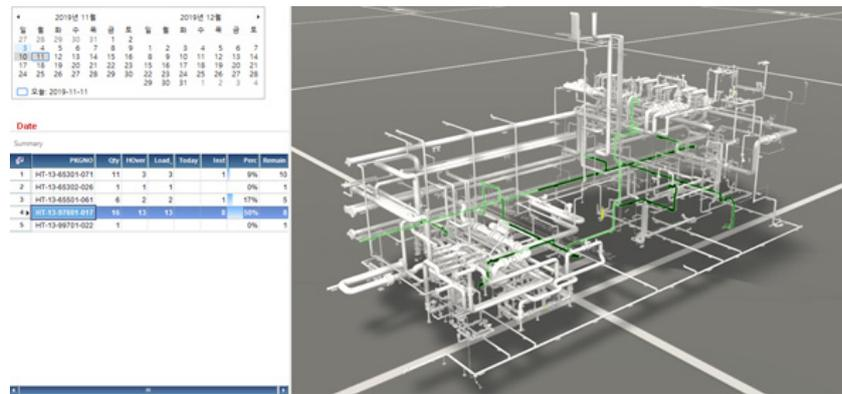
(b) 3D CAD pipe model with identical package for pipe flushing
