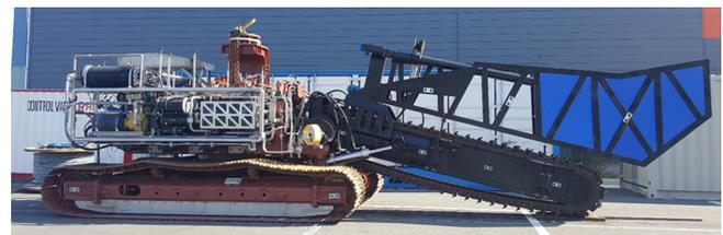
**Fig. 1** Underwater construction robot URI-R
