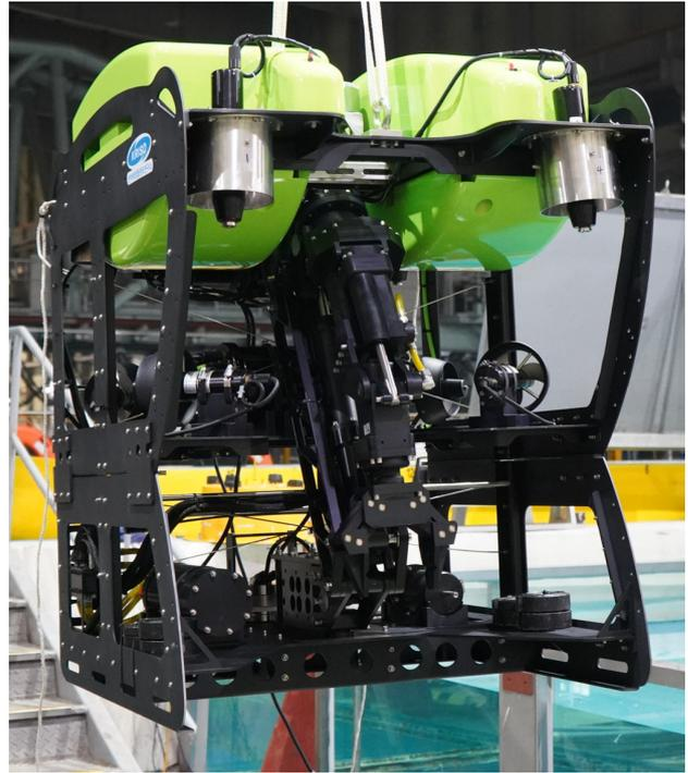
**Fig. 1** Underwater robot with ECA ARM 7E Mini
