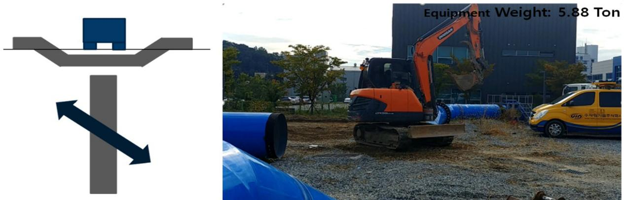
Fig. 11 test result of unbalanced load (45° direction) testing using weight of 5.88 t pork crane at buried pipe
