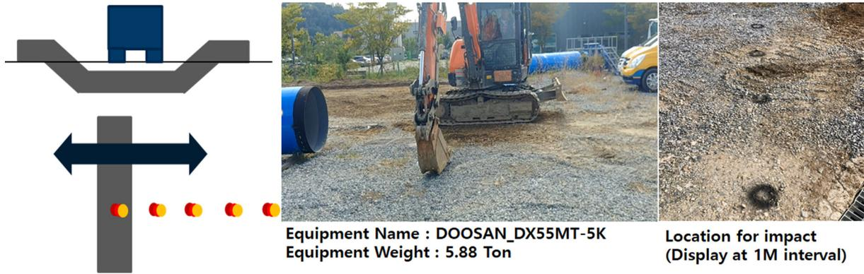
Fig. 13 Test of moved impact load on buried pipelines
