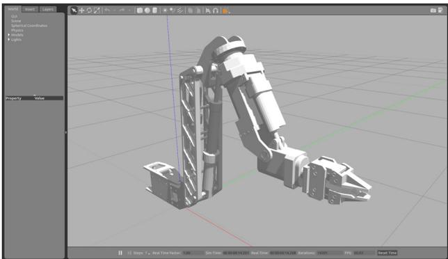
Fig. 7 Gazebo simulation with the ECA ARM 7E Mini
