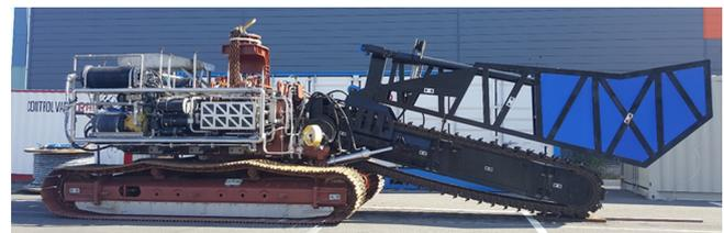
**Fig. 1** Underwater construction robot URI-R
