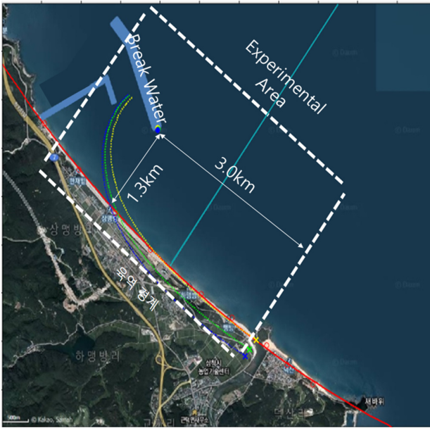
Fig. 5 Object area of hydraulic model experiment (4.0 km × 2.8 km)
