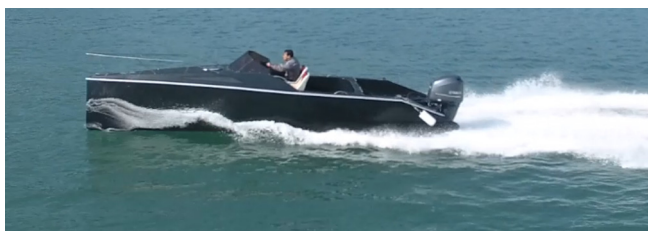
Fig. 4 Sea trial for measurement of speed, WPH (V=35knots)
