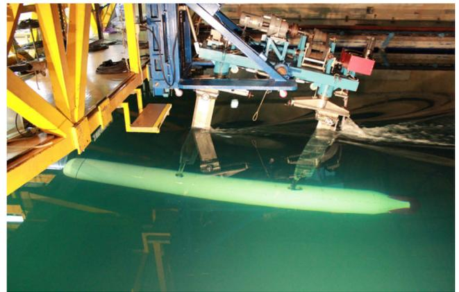
Fig. 4 Photograph of static elevator with angle of attack test
