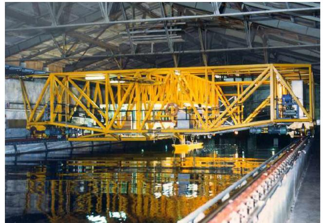
**Fig. 2** Towing tank of KRISO
