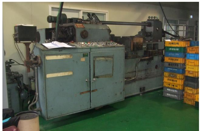
**Fig. 3** Appearance of friction welding machine(Model: FF-60 II M-S1)
