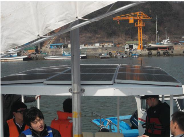
**Fig. 6** Actual image to show the photovoltaic panels used for photovoltaic hybrid generating system
