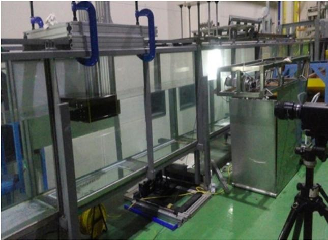
Fig. 3 Experimental set-up in 2-D wave tank
