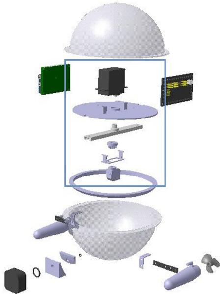
Fig. 9 Designed buoy robot-kit (disassembled)
